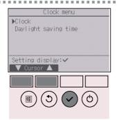
Move the cursor to "Clock" with the F1 or F2 button, and press the SELECT button.
