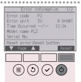
Press the F4 button or the ON/OFF button to reset the error that is occurring.
