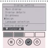
Move the cursor to "Design" with the F1 or F2 button, and press the SELECT button.
