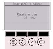
This screen allows the user to wipe the touch panel for 30 seconds without accidentally changing the settings.
