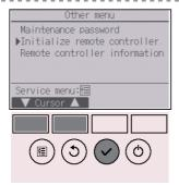
Move the cursor to "Initialize remote controller" with the F1 or F2 button, and press the SELECT button.
