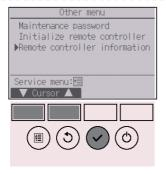
Move the cursor to "Remote controller information" with the F1 or F2 button, and press the SELECT button.
