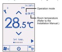
Press the ▼ button to decrease the preset temperature, and press the ▲ button to increase.
