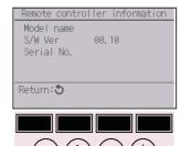
The model name, software version, and serial number of the remote controller in use can be checked.
