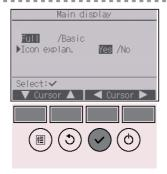
Select "Icon explan." with the F1 or F2 button, select the desired setting "Yes" or "No" with the F3 or F4 button, and press the SELECT button.
