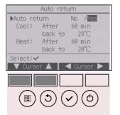
The screen to make the settings for the automatic return to the preset temperature will appear.
