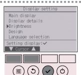
Move the cursor to "Brightness" with the F1 or F2 button, and press the SELECT button.
