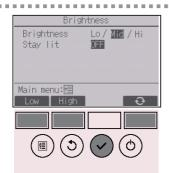
Adjust the brightness with the F1 or F2 button. "ON" or "OFF" can be selected for the "Stay lit" setting with the F4 button.
