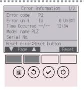
Error code, error unit, refrigerant address, unit model name, date and time on which an error occurred, and serial number will appear.
