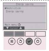
Move the cursor to "Restriction" with the F1 or F2 button, and press the SELECT button.
